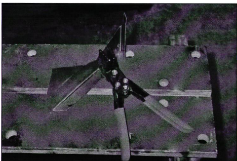
Patch with flanges formed
